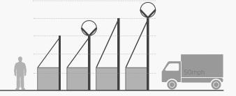
TERRABLOCK XV provides anti-climb protection, vehicle mitigation tested to M50P1 and can be enhanced with intrusion detection and deterrents. Developed and tested over a 5 year period, XV can be deployed in urban or remote environments to protect critical infrastructure and commercial operations.
