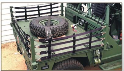
Easy removable set of flexible drop sides of the loading platform for transportation military equipment or small cargo. Set fits to MILPO special trailer and AERO vehicle.
