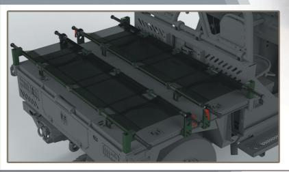
Stretcher holders mounted on the loading platform of the AERO vehicle. For two stretchers compliant with NATO STANDARD.
