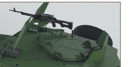
Medium 360 degree turret with bearing. Electric or manual drive with handle for right or left-handed. Armoured shields. Large pintle.
