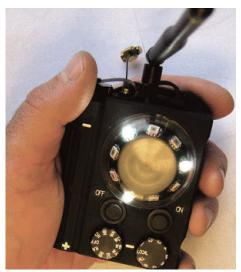
The Airfield beacons uses a UHF transceiver programmed with seven discrete channels. There are three modes: continuous at medium power; continuous at high power and 1 Hz flashing on high power.
